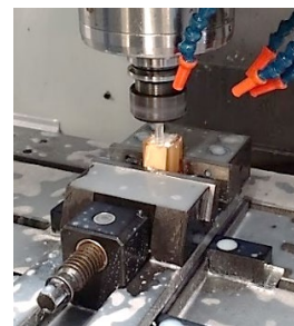
Figure 1. Embedded Macor ® block during machining.
